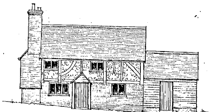
Timber framed, ragstone panels, tiled roof. Added chimney. Ground floor rebuilt in brick. Timber & tiled porch. Weatherboarded & tiled addition. NB First Floor was rendered over with timbers painted on it - not shown. EAST FRONT IN 1878
