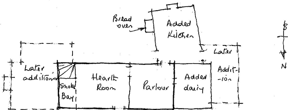
A late 16 C. 2 bay house with end smoke bay, added bays and later additions. Timber framed with gabled tiled roof, the additions of stone. Square panels, straight down braces.
